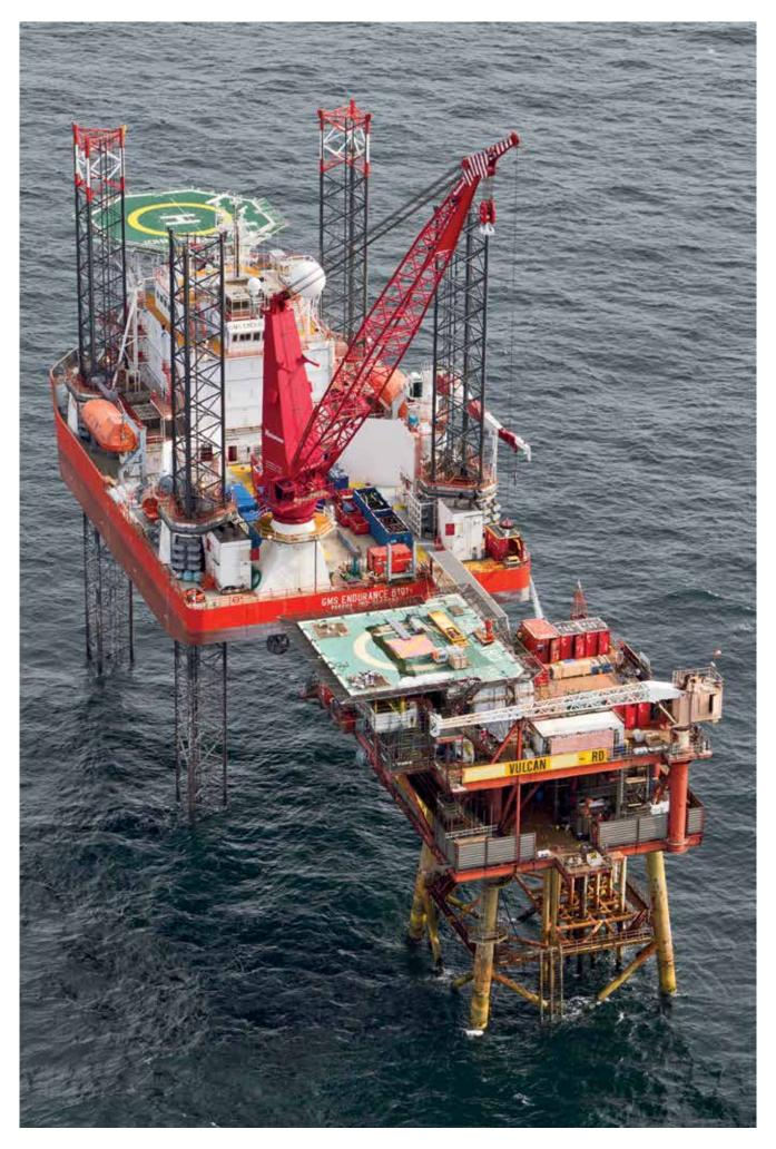
The business model is centred on a commitment to providing a flexible and cost-effective solution for customers operating in the offshore oil, gas and renewable energy sectors using a modern fleet of self-propelled Self-Elevating Support Vessels (SESVs).
